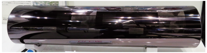
DLC-coated gravure cylinder instead of chrome plating used for printing tests
