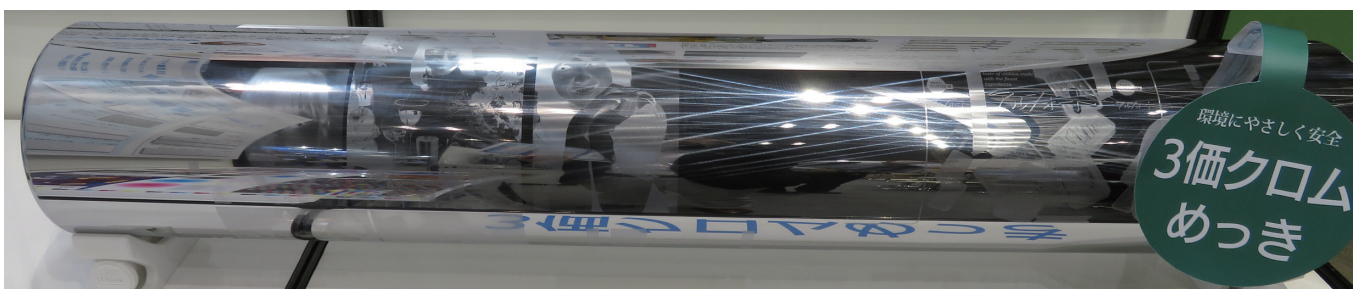
A nearly finished gravure printing cylinder produced with trivalent chromium-based plating process
