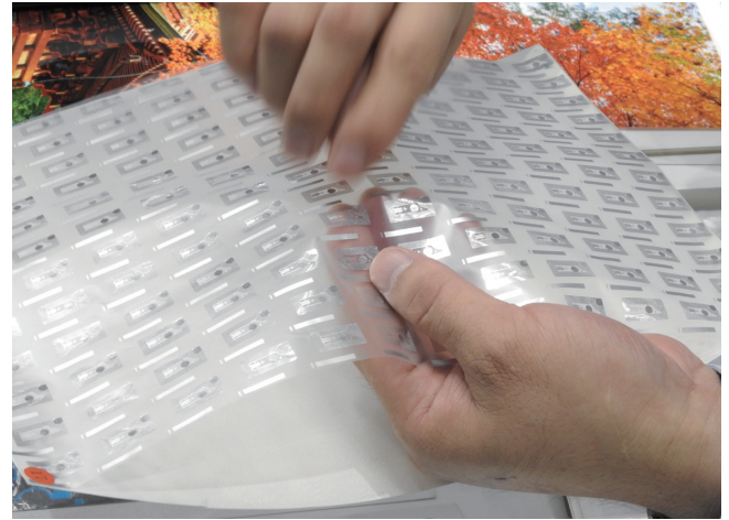
Samples of RFID's antenna circuits printed by use of INHON Laser's gravure cylinders
